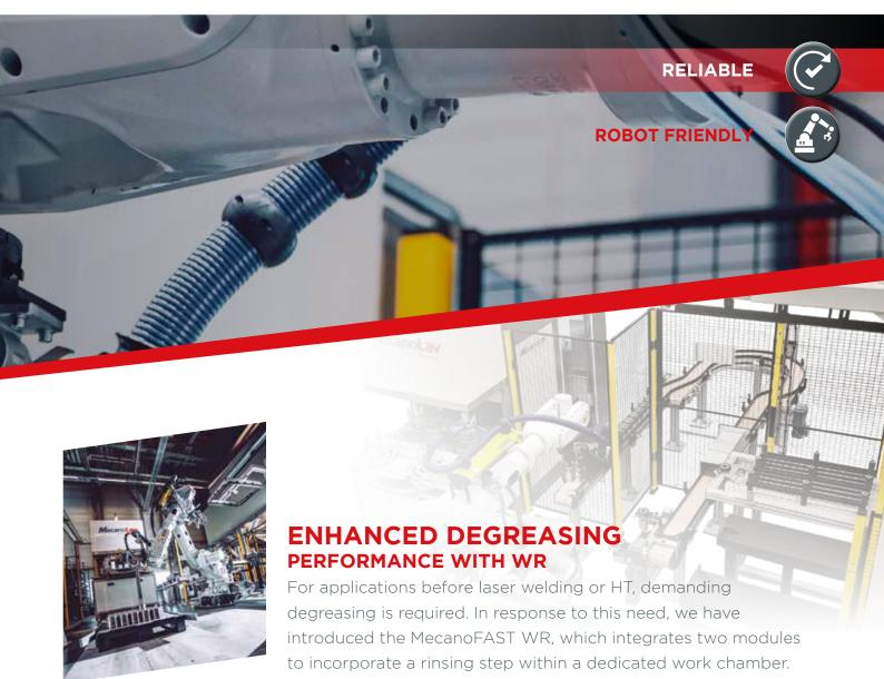
This technology guarantees no fluid transfer from the first to the second unit, thereby prolonging bath lifespan and providing optimal and repeatable cleaning results.
