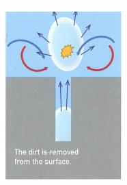
The asymmetrical change of volume creates a pumping effect ensuring the exchange of media in capillaries and holes helping to remove impurities.
