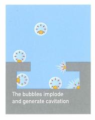
Due to the isostatic distribution of pressure change in the cleaning fluid, Cyclic Nucleation is highly effective in cleaning difficult geometries like undercuts and narrow channels.
